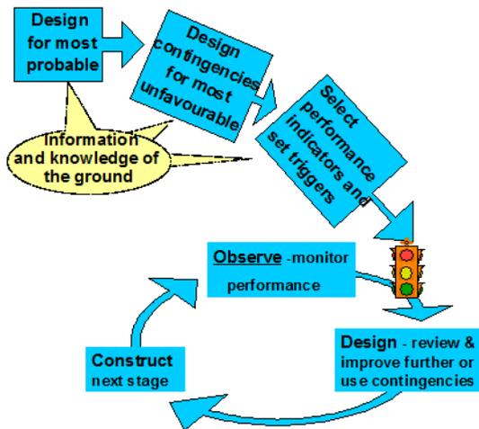
Figure 1 The Observational Method design process
